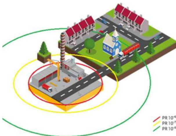
Figure 3-1 Example safety zones including the PR-contour 10^{-4} , 10^{-7} and 10^{-8} (for illustration only)
